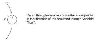
The examples we have seen so far are the *current source* in electrical systems, and the *force source* in mechanical systems.
