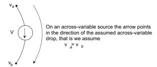
The examples we have seen so far are the *voltage source* in electrical systems, and the *velocity source* in mechanical systems.
