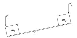
$m_1$  and  $m_2$  are not independent energy storage elements because  $v_1 \propto v_2$  and therefore their energies are algebraically related.
