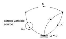
Using impedances, redraw the graph combining the inertia and the spring into a single impedance  $Z_2$ :
