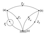
**Step 1:** Write node equations for each node (except the reference node) - let f be a generalized through variable.
