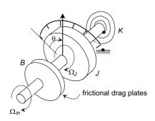
Find the transfer function relating the displacement of the indicator  $\theta$  to the input angular velocity  $\Omega_{in}$
