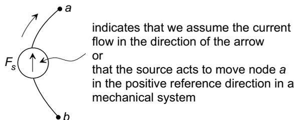
When we draw a branch on a graph we make the assumption that  $P > 0$ , that is that power is flowing into the element. There are in fact two arrows implicit on each branch: one representing the assumed across-variable drop, and a second representing the assumed through-variable direction. If  $P > 0$  (power is flowing into the element), the two arrows are in the same direction. For example, consider a capacitor
