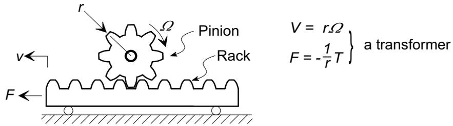
It can be seen that the linear velocity of the rack is proportional to the angular velocity of the pinion. Similarly the force needed to balance the torque applied to the pinion is proportional to the torque. The rack and pinion is therefore a lossless *transformer*.
