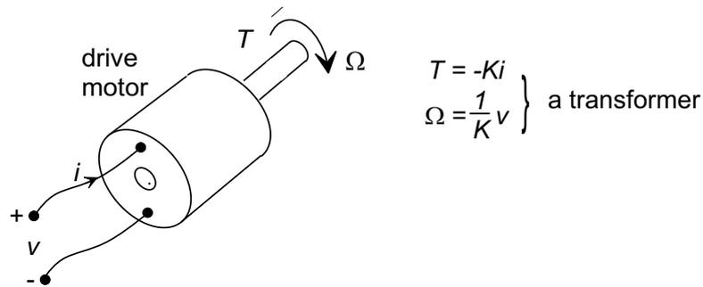
In the dc motor the torque produced is proportional to the current flowing, while the back emf produced is proportional to the angular velocity of the shaft. The motor is a lossless *transformer*.
