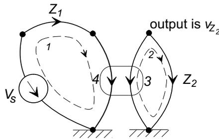
The transformer provides the constraints
