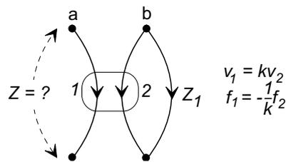
Let an element (or system) with impedance  $Z_1$  be connected across a transformer as shown, then the impedance seen from side 1 of the transformer is
