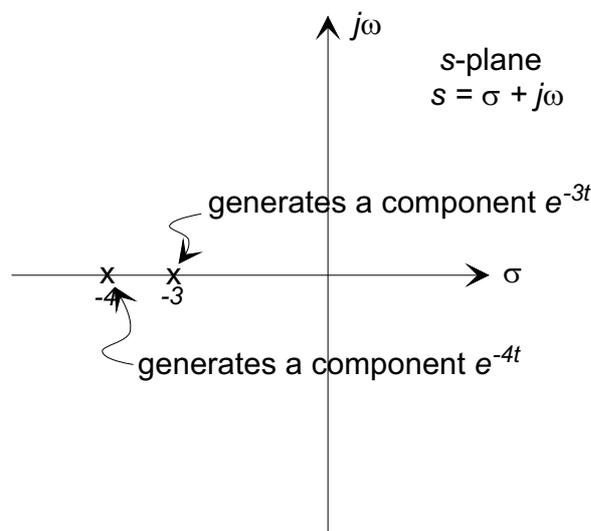
The homogeneous response components are therefore  $y_1(t) = C_1 e^{-3t}$  and  $y_2(t) = C_2 e^{-4t}$ , where  $C_1$  and  $C_2$  are defined by the initial conditions.
