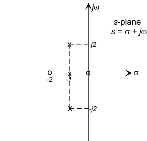
and the modal components are (1)  $Ce^{-t}$  (corresponding to the pole at  $s = -1$ ), and (2)  $Ae^{-t} \sin(2t + \phi)$  (corresponding to the complex conjugate pole pair at  $s = -1 \pm j2$ ), and where the constants  $C$ ,  $A$ , and  $\phi$  are determined from the initial conditions.
