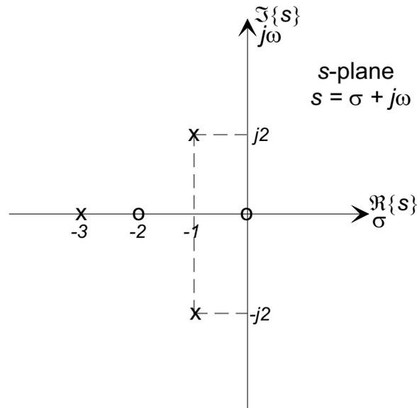
where the pole positions are denoted by an **x**, and the zeros are drawn as an **o**. The figure shows zeros at  $s = 0, -2$ , and poles at  $s = -3, -1 \pm j2$ .
