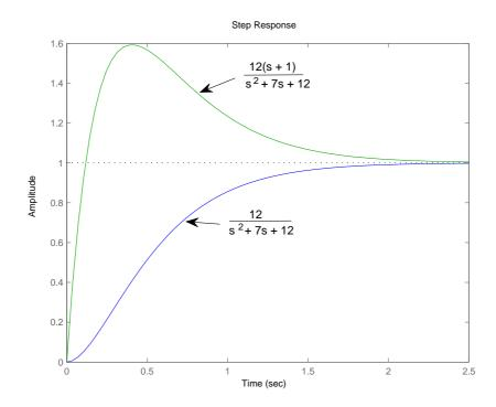
Note the overshoot caused by the zero, but that the overshoot is not oscillatory. Clearly the rise-time  $T_R$  is much shorter for the system with the zero.
