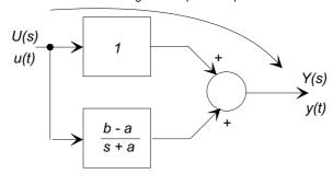
showing a direct *feed-through* of the input into the output. In other words, when the order of the numerator is the same of the denominator the *input will appear directly as a component* of the output.
