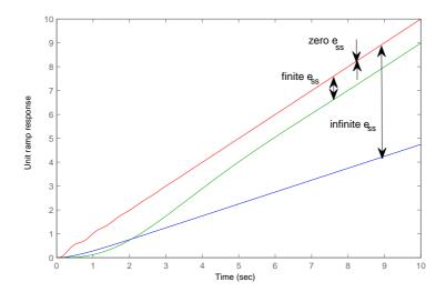
The above figure shows three responses to a unit ramp input r(t) = t. In one case there is no steady-state error - as t becomes large, the response follows the input exactly. In the second case there is a finite steady state error, the response has unit slope but exhibits a constant offset from the input. The third case shows a response in which the error is growing without bound, and the steady-state error is infinite.
