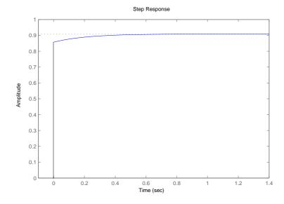
The step response is shown below – note the initial transient caused by the direct feed-through.
