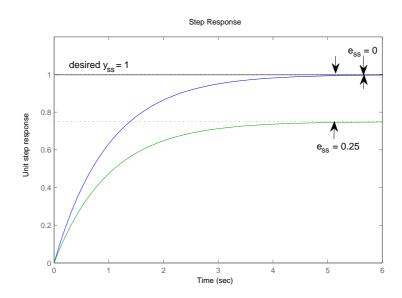
The above figure shows the response to a unit step. One response exhibits  $e_{ss} = 0$ , while the other shows a constant steady-state error.
