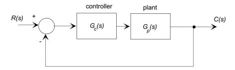
Combine the two cascaded blocks to form a single forward transfer function  $G_f(s) = G_c(s)G_p(s)$
