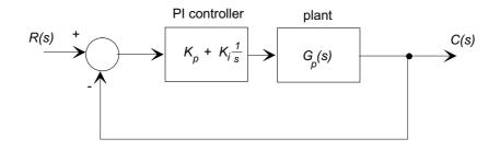
For a PI controller, the transfer function is
