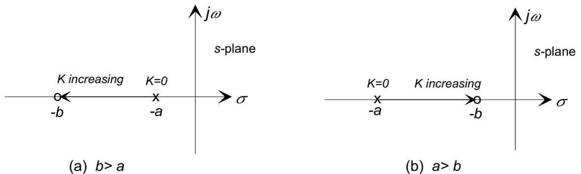
While the root locus always *originates* at the pole and *terminates* at the zero, if  $b > a$  the closed-loop pole will move to the left, while if  $a > b$  the pole will move to the right. In addition we can note:
