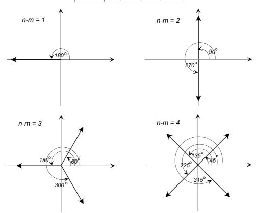
As the gain K becomes large, n-m branches of the root locus diverge away from the origin and approach n-m radial asymptotes, at angles  $\theta_k = (2k+1)\pi/(n-m)$ , for  $k=0\dots(n-m-1)$ .
