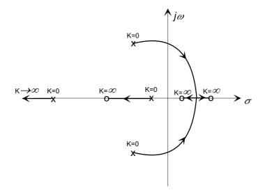
where we note that branches must originate from the complex conjugate pole pair and terminate on the r.h. plane zeros.
