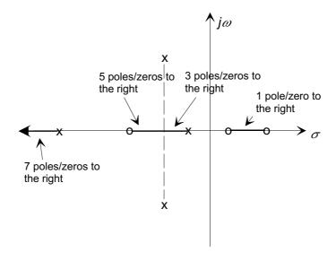
Since we know that (1) branches must originate from open-loop poles, and (2) terminate on open-loop zeros or go to infinity, we have enough information to sketch the *form* of the root locus:
