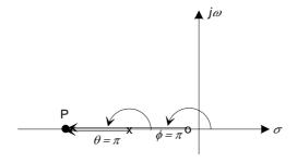
(c) A complex conjugate pole or zero pair contributes a total of zero  $(2\pi)$ to the angle condition along the real axis.
