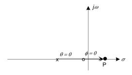
(b) Poles and zeros on the real axis that lie to the right of the point s contribute  $\pm \pi$  to the angle condition.
