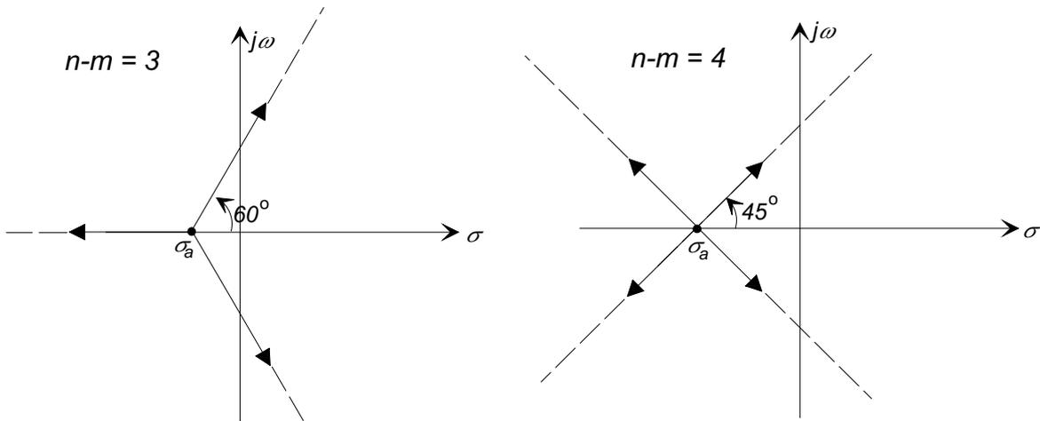
The root locus sketching rule, for constructing the locus of a system with  $m$  open-loop zeros, and  $n$  open-loop poles, for large values of gain  $K$  is therefore:
