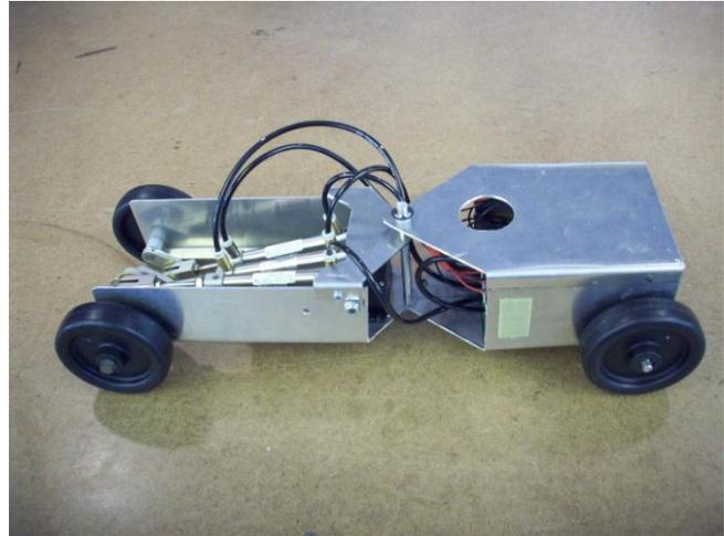
**The valves can be use to extend two of the pistons and retract the other. Then one can be extended while the other two are retracted. This scheme can be repeated through six different states. A firing sequence I propose is.**
