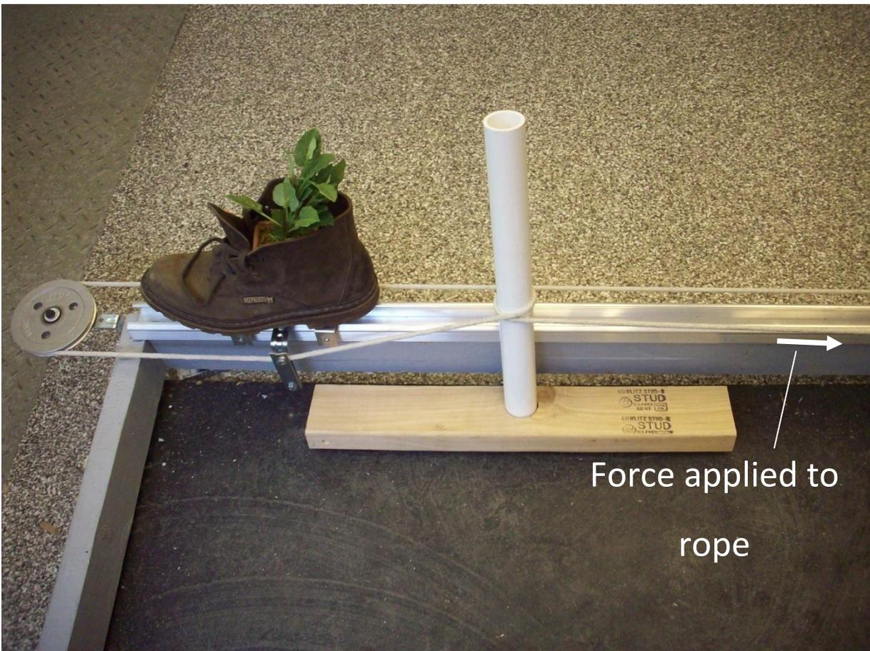
5. (10 points) A person wishes to keep a rope in a fixed location despite a force applied to the rope by another person seeking to move it. They propose to wrap the rope once around a PVC pipe (as shown above). The end of the PVC pipe is placed within a hole in a 2 in by 4 in piece of lumber which is then pinned in place (the pin is not shown above).
