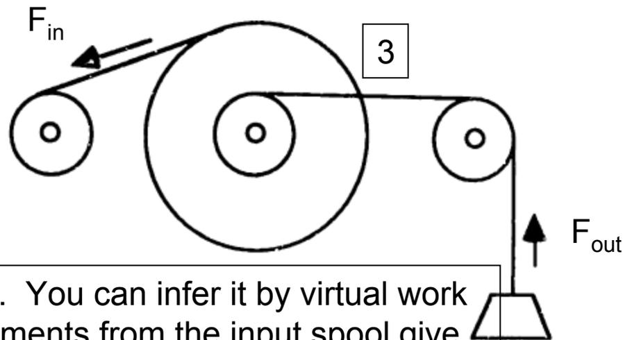
The answer is 3. You can infer it by virtual work -- large displacements from the input spool give only small displacements onto the output spool
