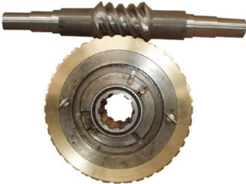
We really didn't discuss this, so I think it's not testable. But the "enveloping" feature is the curvature of the faces to accomplish more tooth to tooth contact. You should be able to see this gear is multi-threaded because the thread on the worm gear extends across such a long distance as it moves 180 deg across the face. There are clearly two threads interleaved.
