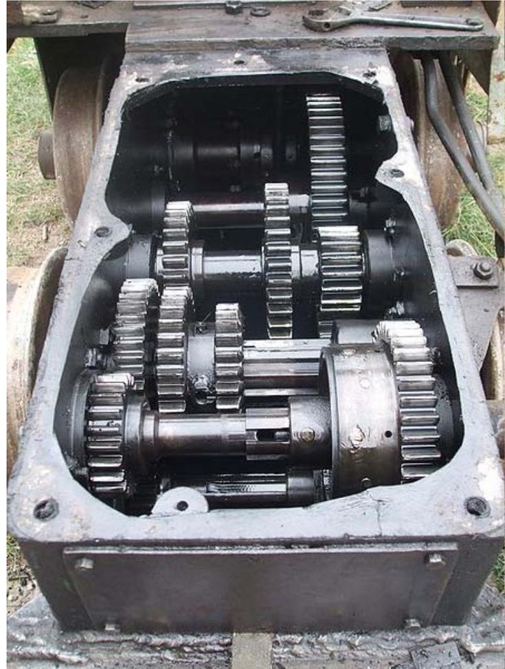
The key thing is that the total reduction ratio is a product of the ratios of the two mating pairs.
