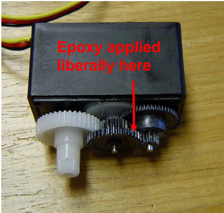
The gears nearest the output shaft will fail since they experience the highest loads. The mode for Delrin gears is most probably in bending or “stripping”. I would estimate that the smaller gear (black in the photo) will fail rather than the white one since it has a narrower base and so a lower Lewis factor.
