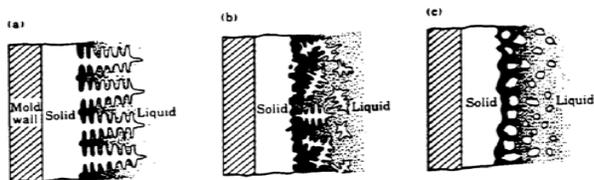
Schematic illustration of three basic types of cast structures
