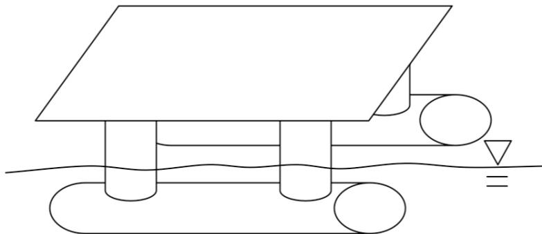
The diameter of the uprights is 10 m, and that of the pontoons is 10 m. The length of the pontoons is 100 m. The added mass of the uprights is negligible compared to that of the pontoons.
