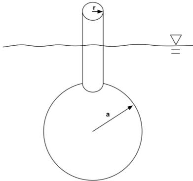
The added mass of the cylinder is negligible compared to that of the sphere:
