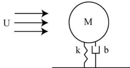
Figure 1 – Flexibly -mounted cylinder in a steady flow
