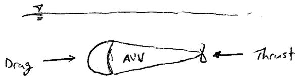
At steady speed, thrust = drag
