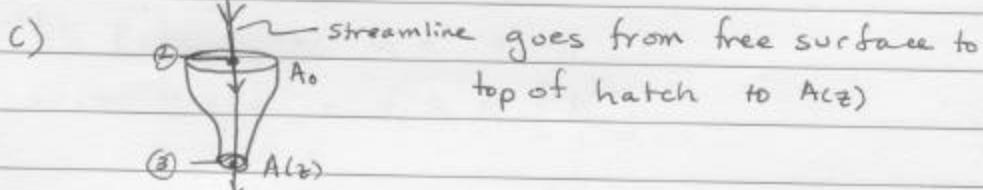
$$P_1 + \frac{1}{2} \rho V_1^2 + \rho g z_1 = P_2 + \frac{1}{2} \rho V_2^2 + \rho g z_2 = P_3 + \frac{1}{2} \rho V_3^2 + \rho g z_3$$
