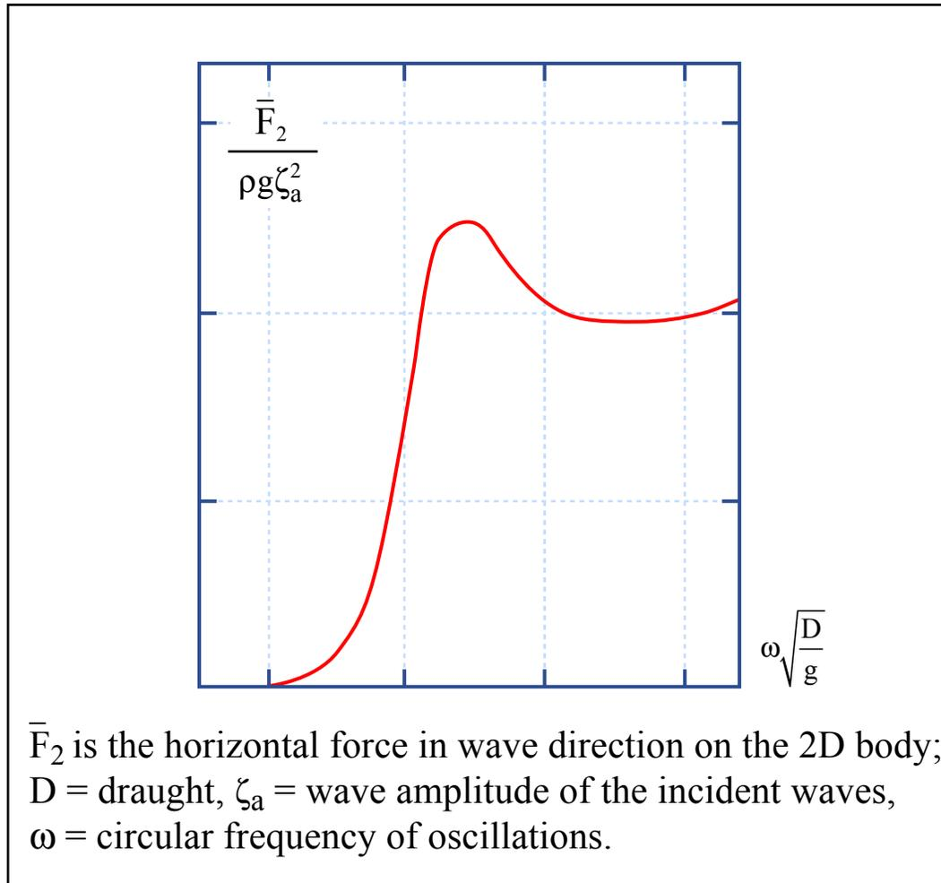
F2 is the horizontal force in wave direction on the 2D body
