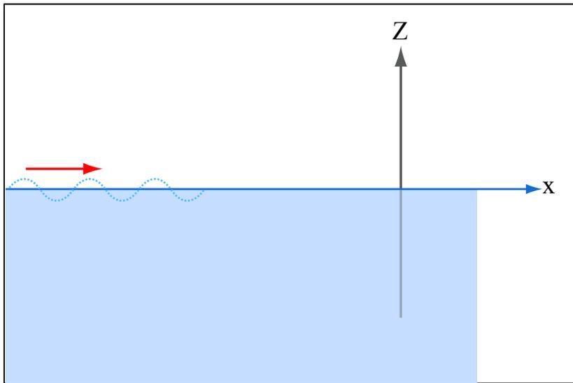
Diagram showing drift forces and incident waves on a vertical wall, Z. Image by MIT OpenCourseWare.
