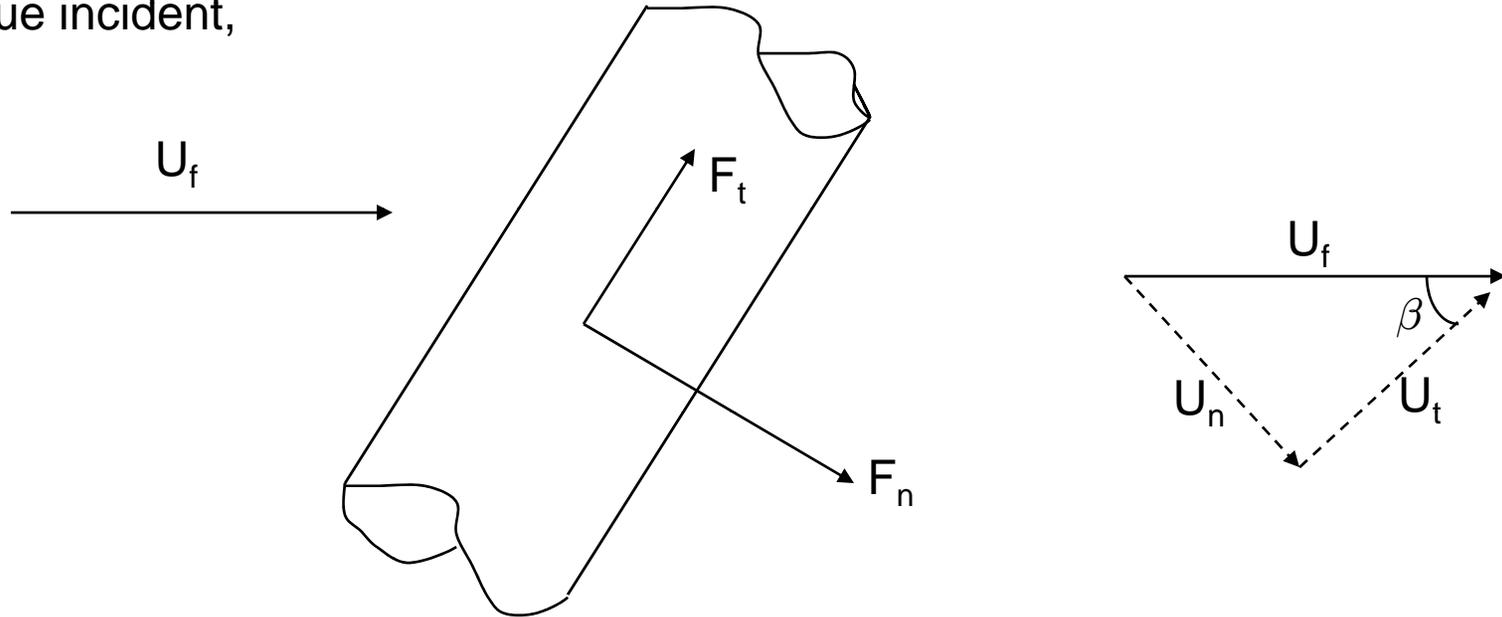
Normal component  $U_n$  causes flow separation drag, tangential component  $U_t$  causes frictional drag
