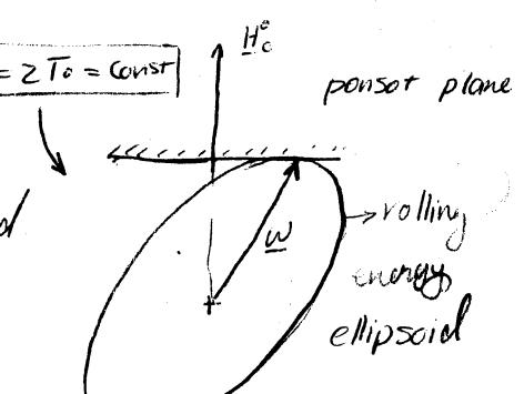
$\Rightarrow$  trajectories (orbits) of Euler's spinning top form curves on the energy ellipsoid
