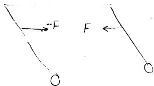
$$F = -c \frac{d}{dt} [h(\sin \varphi_2 - \sin \varphi_1) \dot{\varphi}_2 - h(\cos \varphi_2 - \cos \varphi_1) \dot{\varphi}_1]$$
