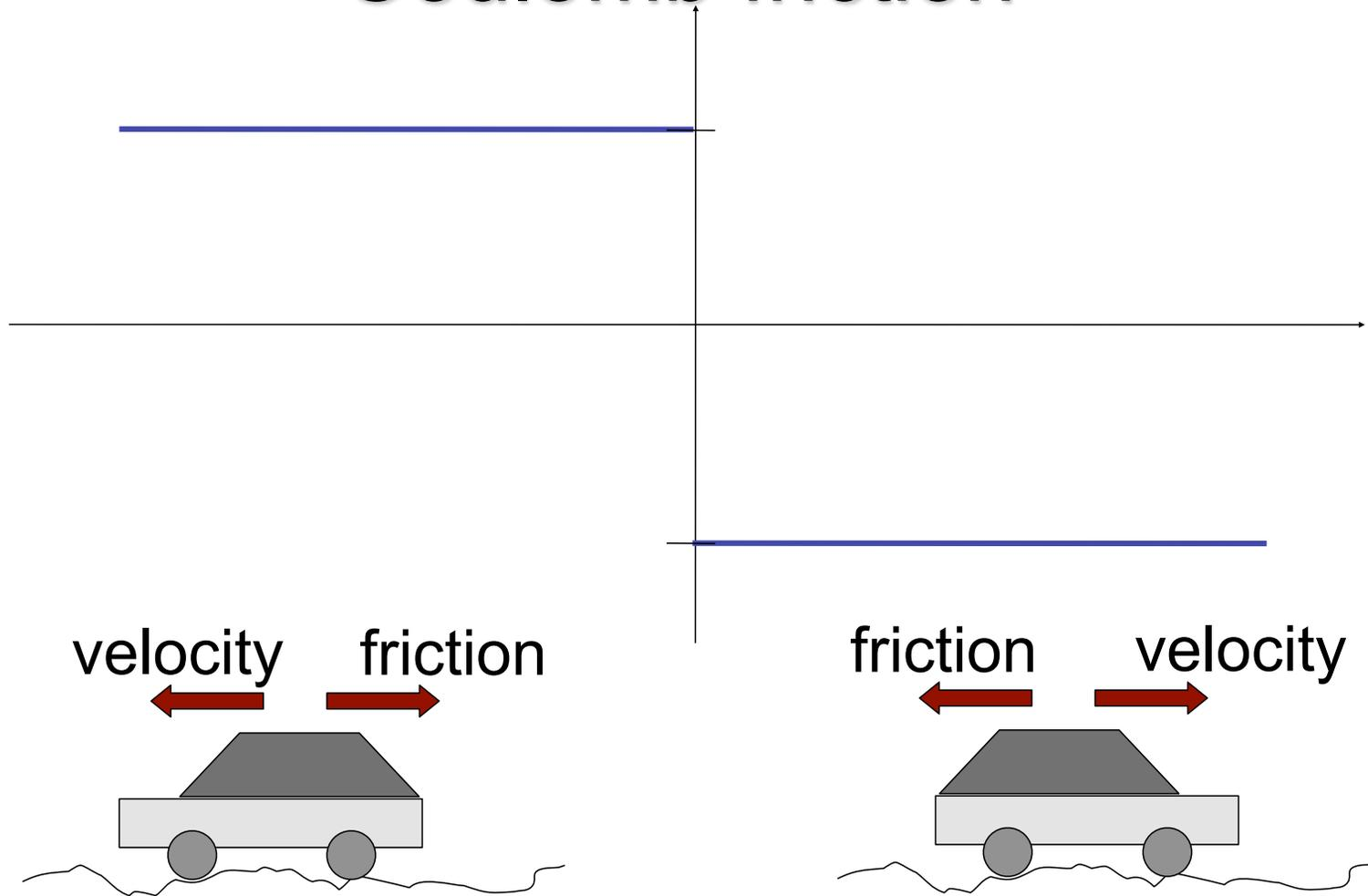
*Coulomb* friction is in opposite direction to the velocity; the magnitude of the friction force is independent of the magnitude of the velocity
