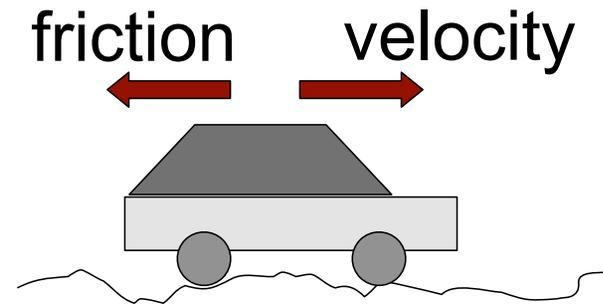
*Viscous* friction is in opposite direction to the velocity; the magnitude of the friction force is proportional to the magnitude of the velocity
