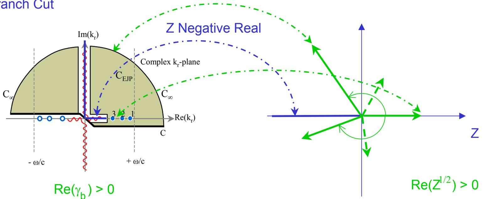
EJP Branch Cut: Bottom field decaying for all  $k_r$  => Physical Riemann Sheet
