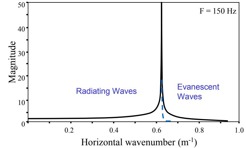
Magnitude of the depth-dependent Green's function for point source in an infinite medium. Solid curve:  $z - z_s = \lambda/10$ ; dashed curve:  $z - z_s = 2\lambda$ .
