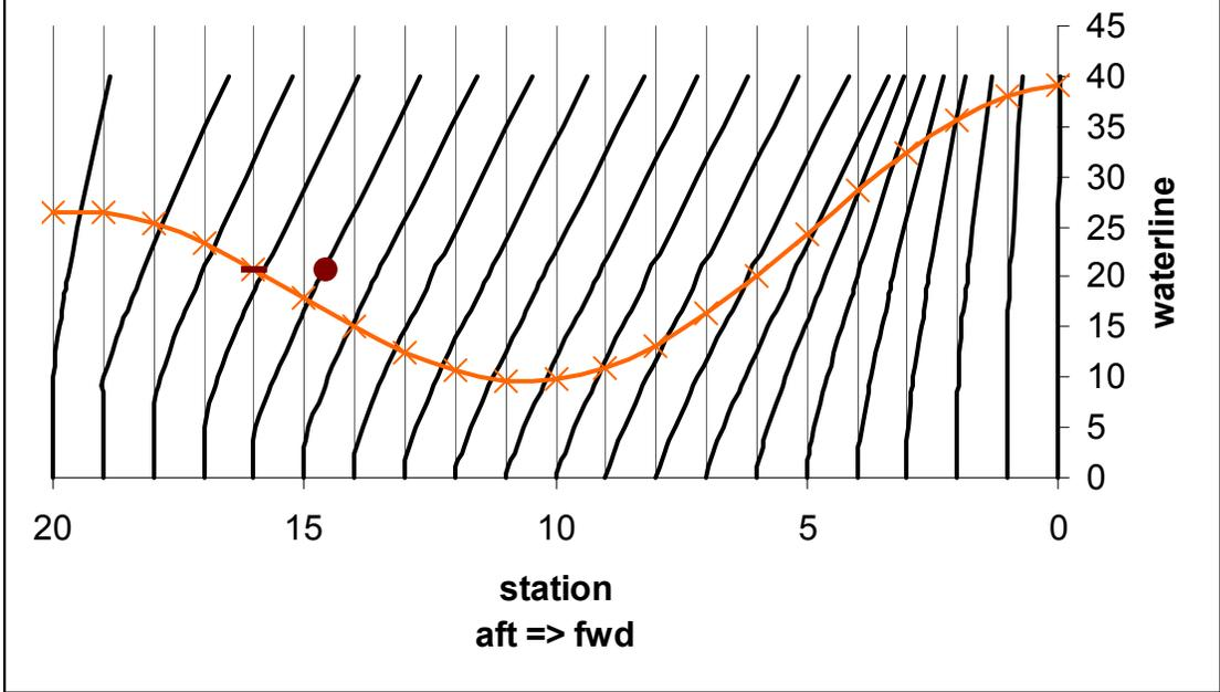
for example: after some iterations a draft and trim is determined that has the following buoyancy per length distribution:
