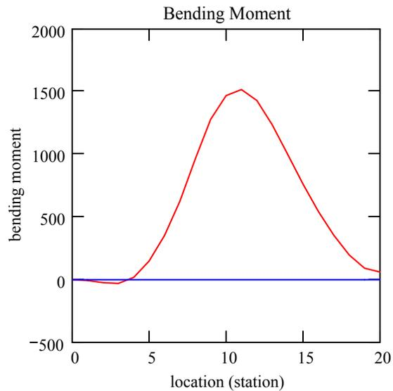
as a check on achieving a true "balance", the shear force and bending moment should be zero at the end ( $x_s = 20$  station). The above data is close but there is a relatively small remainder.
