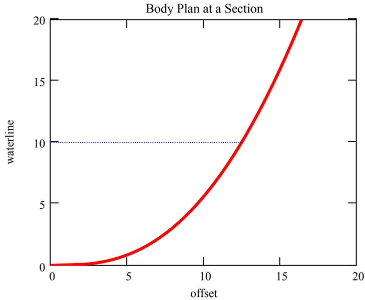
The section area is the area below each waterline. The curve of area below the respective waterline is the section area or Bonjean curve.
