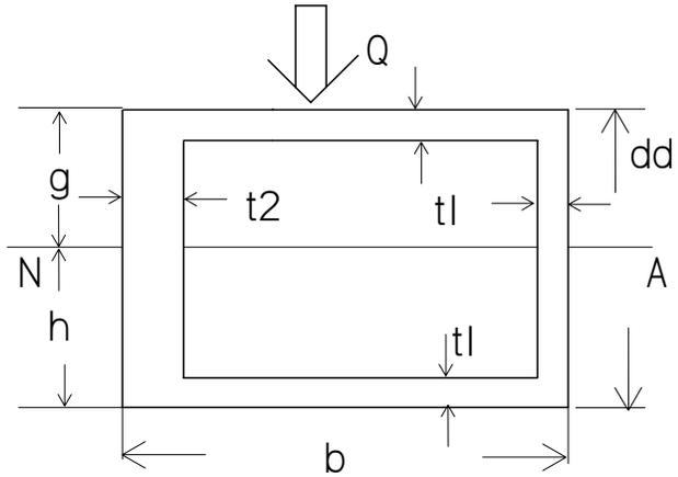
reference baseline, h is distance between NA and lower segment; g = dd - h is distance to top segment
