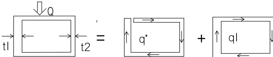
$q^*$  is the shear flow we have developed to date opening the section and
