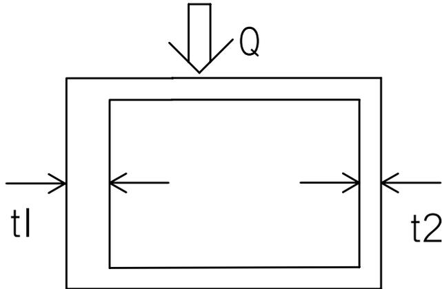
Shear load is applied such that (pure) bending occurs
