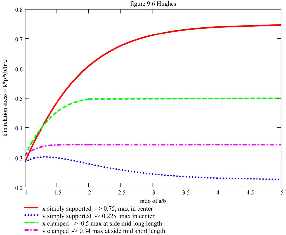
$M_x$  is max ( $k = 0.5$ ) at  $x = a/2$ , i.e. at ends of short side, middle of long side
