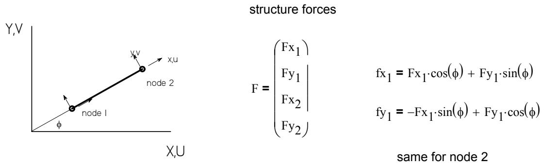
N.B.  $\phi$  is the angle measured CCW from the structure X to the element x coordinate direction
