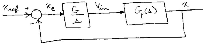
The controller for this loop is an integral controller  $G_c(s) \equiv G/s$ , where  $G$  is an adjustable gain associated with the integrator.
