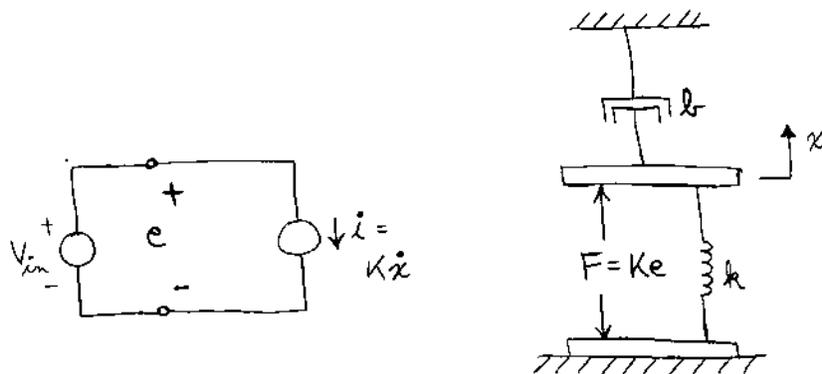
Here, the piezoelectric actuator is modeled internally as a dependent force source  $F(t)$  in parallel with a spring  $k$ . The force depends linearly upon the input voltage as  $F(t) = Ke(t)$ , where  $K$  is a scale factor with units of  $N/V$ . The spring  $k$  models the internal stiffness of the piezoelectric actuator. The force  $F$  is applied to the massless upper plate which connects the damper and spring.
