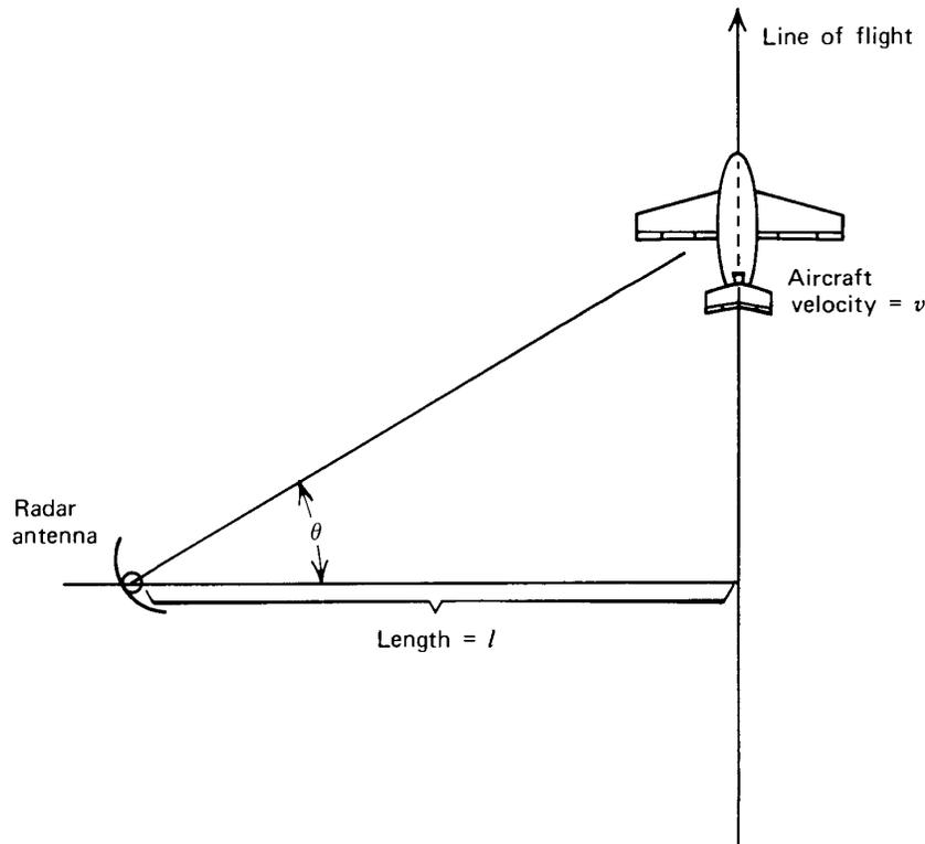
**Figure 3.18** Radar antenna tracking an airplane.
