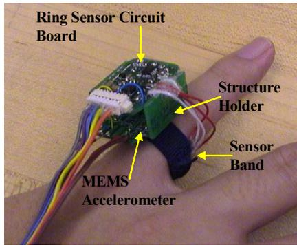
Figure 1 MEMS accelerometer collocated with PPG ring sensor
