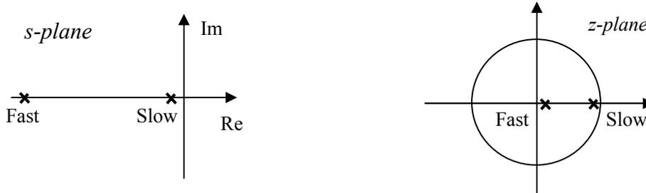
Choose  $\bar{a}$  such that  $p_1 \cong -\bar{a}$ , where  $p_1$  is a slow, stable pole. Using the bilinear transform, this slow pole in the s-plane can be transferred to a fast pole in the z-plane, as shown below. Representing in the z-plane, the transfer function can be truncated; just a few terms can approximate the impulse response since it converges quickly.
