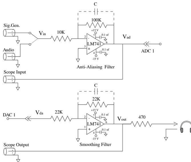
Figure 1: Anti-aliasing and smoothing filter circuit diagram.
