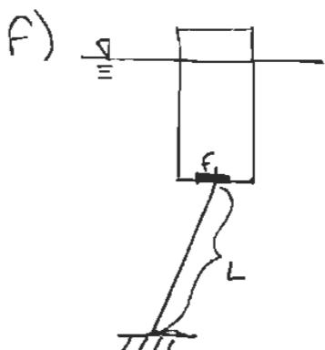
The RESTORING FORCE DUE TO THE CABLE IS  $f_r = k_{11} L \theta = P \sin \theta$
