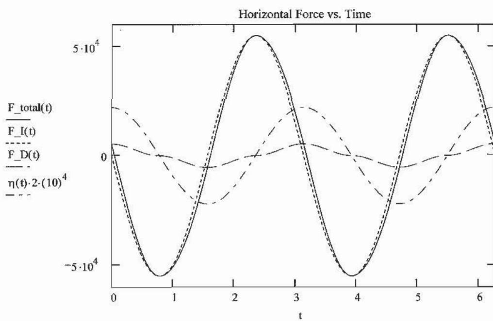
From this plot, you can see that the inertial force component dominates the drag force component in the total force. You can see that the maximum total forces occur when the drag force is zero and inertial force is at the maximum. Wave elevation is included magnified by a factor of  $2 \times 10^4$  so that it shows up on the same graph.
