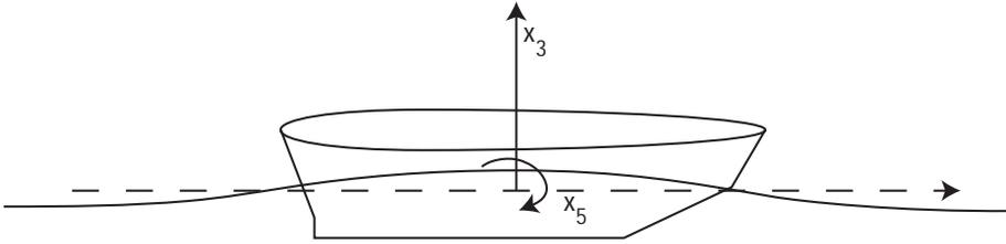
Once we have set up the simple equation of motion for a vessel in heave it is natural to extend this discussion to the coupled heave-pitch equations of motion. Considering a ship floating on the free surface in waves. This ship will naturally heave and pitch due to the incident waves. It is not guaranteed that these two motions will be independent, however. Thus it becomes necessary to consider the motions together.
