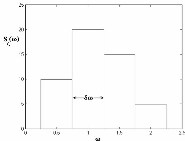
**Figure 1 – Wave energy spectrum**
