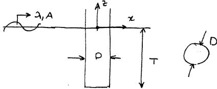
Ambient waves of amplitude A and length  $\lambda$  are incident on the buoy propagating in the positive x-direction.
