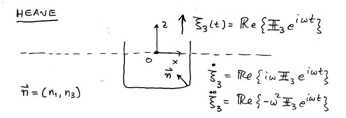
DUE TO THE FORCED OSCILLATION OF THE BODY WITH DISPLACEMENT  $\Xi_3(t)$  A FLUID DISTURBANCE WILL RESULT WITH VELOCITY POTENTIAL
