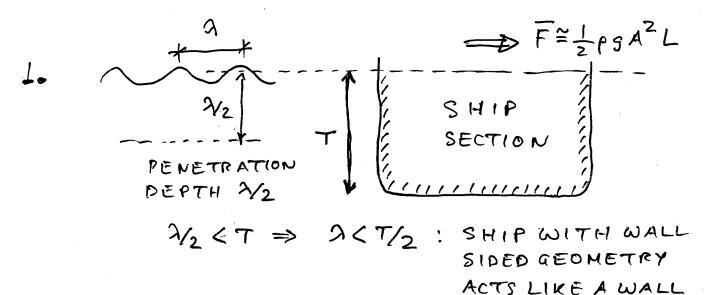
FOR A BARGE LIKE SHIP WITH LENGTH L
