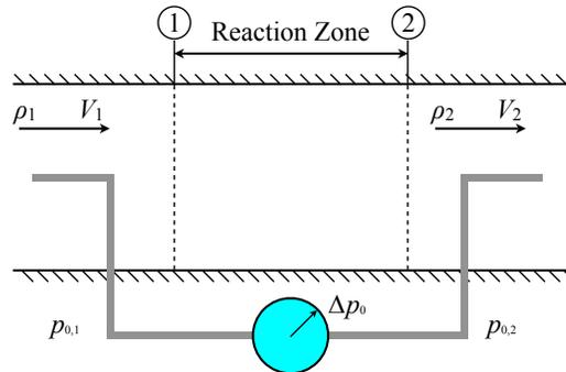
The sketch shows a liquid emulsion (a finely-divided mixture of two liquids) of mean density  $\rho_1$  entering a reaction zone of a constant-area reactor with speed  $V_1$ . The components of the emulsion react chemically, and leave the reaction zone as a liquid at the density  $\rho_2$ . Pitot tubes are installed upstream of the reaction zone. (Pressure inside a pitot tube is stagnation pressure,  $p_0 = p + \frac{1}{2}\rho V^2$ ).
