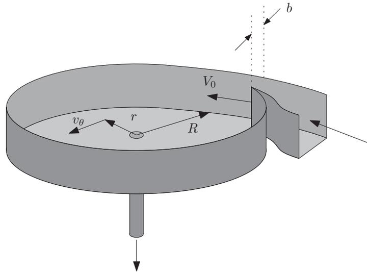
The steady sink flow in the sketch is set up by injecting water tangentially through a narrow channel near the periphery and letting it drain through a hole at the center. The vessel has a radius  $R$ . At the point of injection, the water has a velocity  $V$  and depth  $h_0$ ; the width of the injection channel,  $b$ , is small compared with  $R$ .
