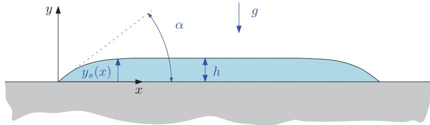
A liquid of density  $\rho$  and surface tension  $\sigma$  has been spilled on a horizontal plate so that it forms a very large puddle whose depth (in the central parts) is  $h$ . Consider the region near the edge of the puddle, which can be viewed to good approximation as two-dimensional. If the contact angle is  $\alpha$ , derive an expression for the shape of the liquid surface  $y_s(x)$ .
