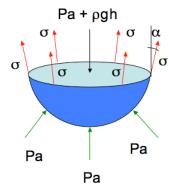
Here too, we could also have performed a force balance and obtain the same result. The force going down is simply the hydrostatic pressure force,  $\pi R'^2(\rho g h + P_a)$ , and the forces going up are the atmospheric pressure force acting on the bottom of the drop, and the surface tension,  $\pi R'^2 P_a + 2\pi R' \sigma \sin \alpha$ . Now, performing a force balance,
