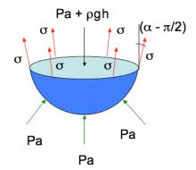
Note that we could also have performed a force balance and obtain the same result. The force going down is simply the hydrostatic pressure force,  $\pi R^2(\rho gh + P_a)$ , and the forces going up are the atmospheric pressure
