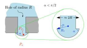
Now, let's use the pressure argument again. From hydrostatics:  $P_i = P_a + \rho g h$ . Also,  $P_o = P_a$ , now calculating the pressure inside the drop from the bottom,  $P_o - P_i = \sigma \left(\frac{1}{R_1} + \frac{1}{R_2}\right)$  From the figure:  $R_1 = R_2 = \frac{R'}{\sin \alpha}$
