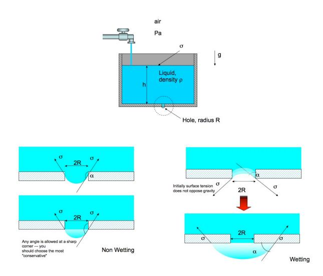
A container is being filled with liquid of density  $\rho$ . A small, sharp-edged hole of radius R penetrates the container's bottom. The surface tension between the liquid and the ambient air is  $\sigma$ , and the contact angle for the air/liquid/container combination is  $\alpha$  (measured from the wall through the liquid to the interface).
