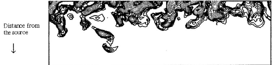
Fig. 9.1. Contours of the kinetic energy on a plane in the flow created by an oscillating grid in a quiescent fluid; the grid is located at the top of the figure. Energetic packets of fluid transfer energy away from the grid region. From Briggs et al. (1996)
