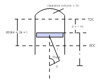
Compression ratio (geometric) -  $C_{R} = \frac{V_{D} + V_{C}}{V_{c}}$
