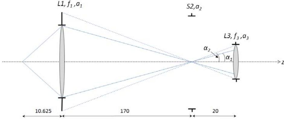
Figure 8: Finding the aperture stop.
