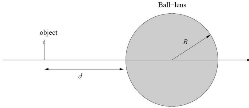
Figure 3: Imaging with a ball lens magnifier.
