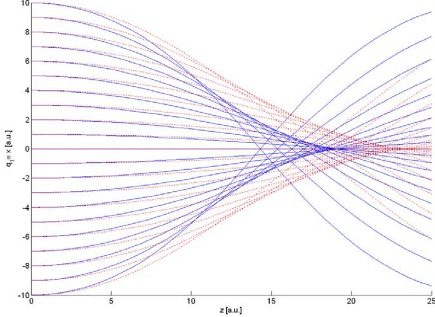
Figure 3: Comparison of quadratic and elliptical GRIN lenses.
