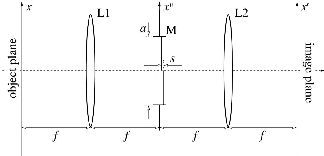
The pupil mask M has aperture  $a = 1\text{cm}$ . Inside the aperture there is a piece of glass of refractive index  $n = 1.5$ . The glass has been partially etched to form a step of height  $s = 1\mu\text{m}$ , and the step is precisely aligned with the optical axis, as shown.
