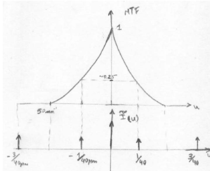
(c) The incoherent transfer function is an autocorrelation of the coherent transfer function. The coherent transfer function in this case is probably a triangle function with half the cut-off frequency.
