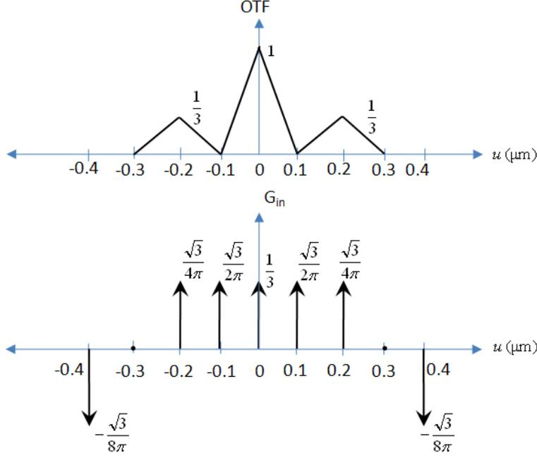
Figure 3: OTF and spectrum of the input signal.
