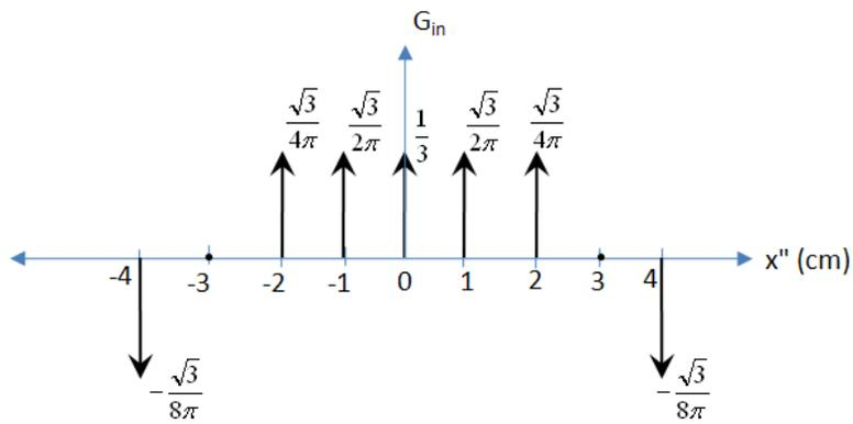
Figure 2: Input signal spectrum.
