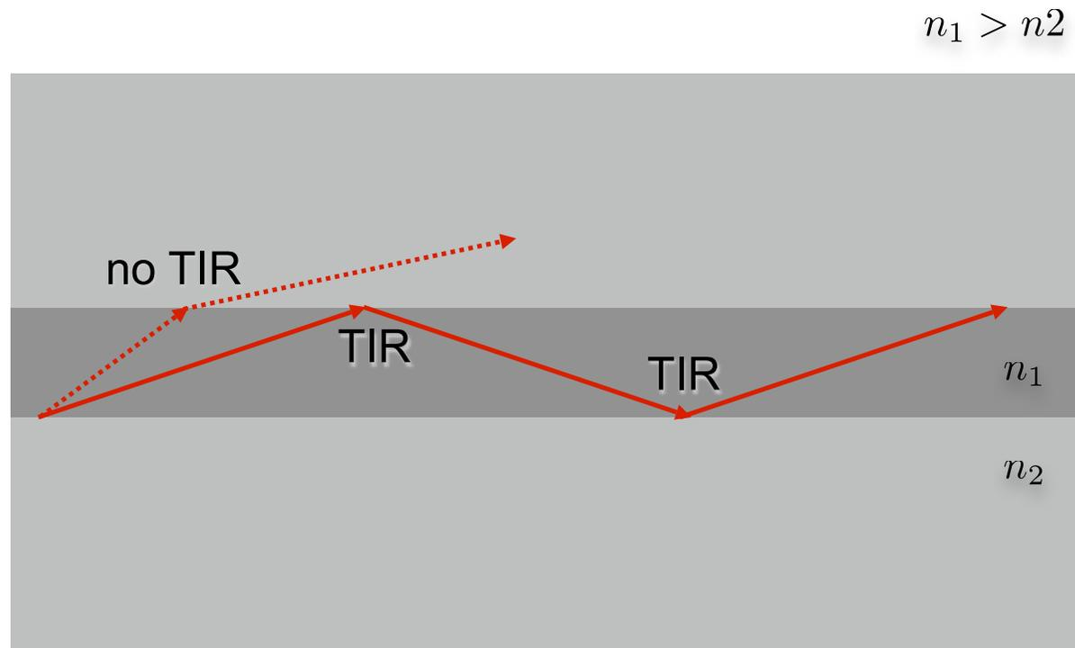
“planar” waveguide: high-index dielectric material sandwiched between lower-index dielectrics
