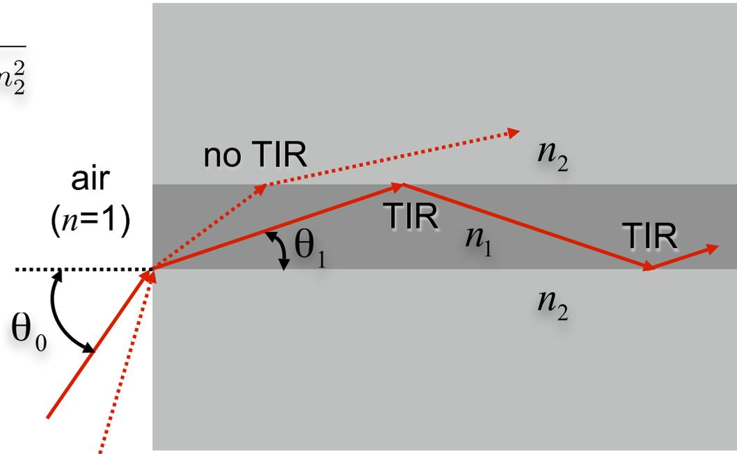
i.e., NA is the incident *angle of acceptance* of the waveguide
