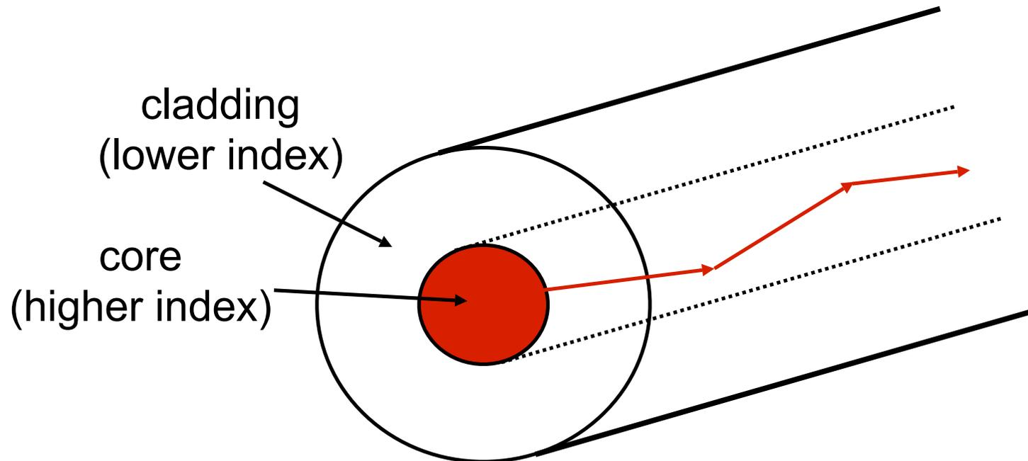
Core diameter = 8-10 $\mu\text{m}$  (commercial grade)
