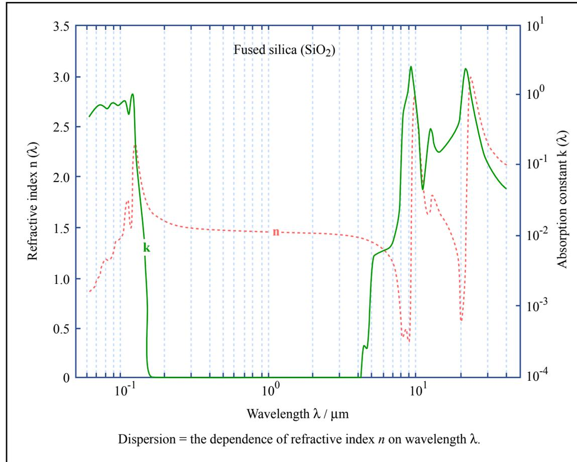
Figure by MIT OpenCourseWare. Adapted from Fig. 2.4 in Bach, Hans, and Norbert Neuroth. *The Properties of Optical Glass*. New York, NY: Springer, 2004.
