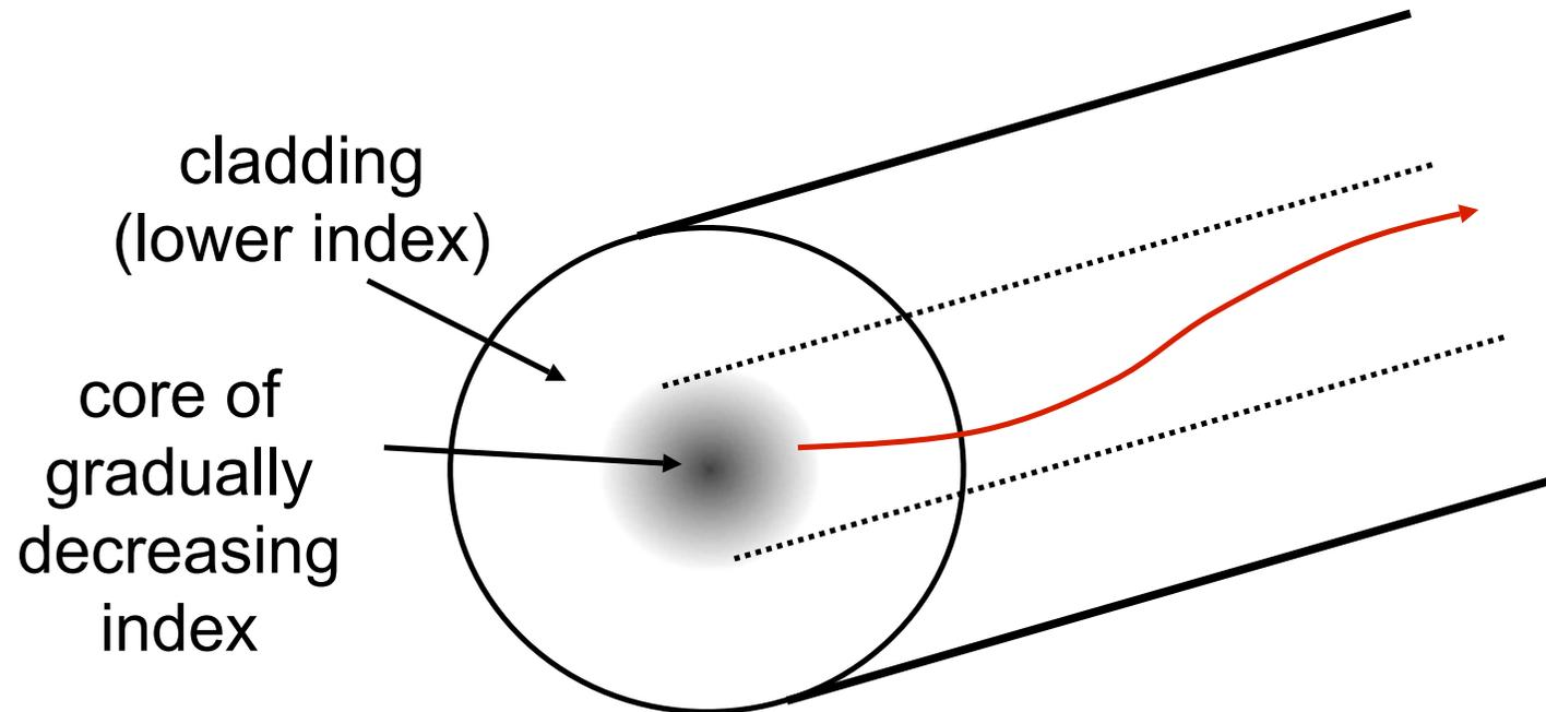
optical rays “swirl” in a helical trajectory
